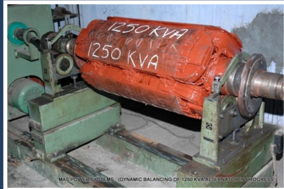
Dynamic Balancing of alternator rotor
