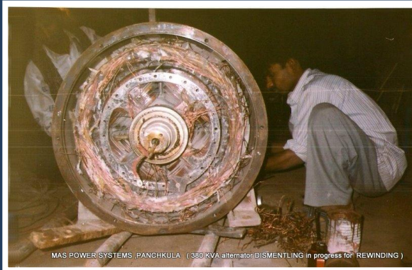
Dismantling of alternator for testing
