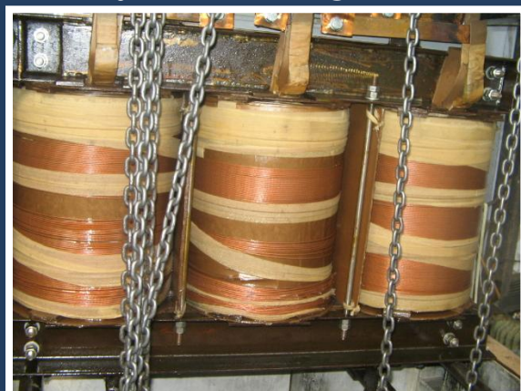
Testing of H.T transformer after rewinding.
